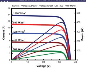
The specifications are obtained under the standard test conditions: 1000W/m2 solar irradiance, 1.5 Air Mass and cell temperature of 25°C. Measurement uncertainty for all panels is 3%. The actual transactions will be subject to the contracts. These parameters are for reference only and it is not a part of the contracts. The technical specifications in this document may vary. For more
