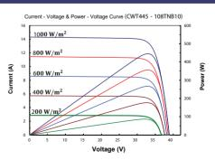
The specifications are obtained under the standard test conditions: 1000W/m2 solar irradiance, 1.5 Air Mass and cell temperature of 25°C. Measurement uncertainty for all panels is 3%. The actual transactions will be subject to the contracts. These parameters are for reference only and it is not a part of the contracts. The technical specifications in this document may vary. For more
